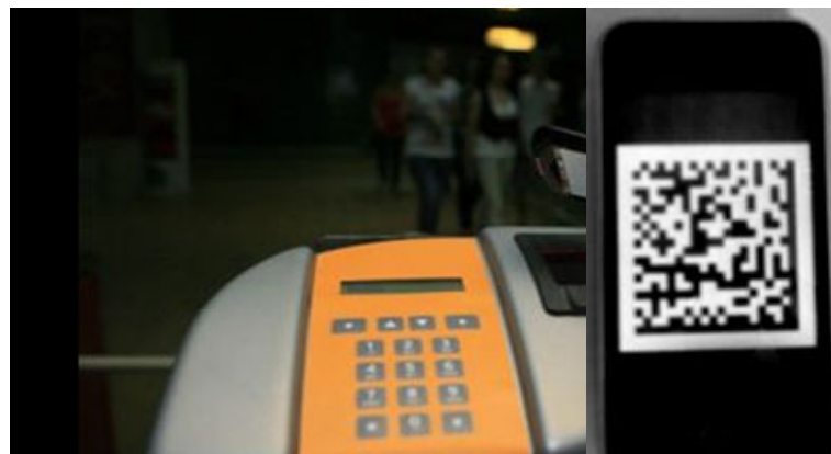
Fig. 1. Presenting a Data matrix 2D barcodes instead of a ticket to the validation device in a subway station – Metrorex Bucharest, Romania
