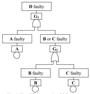
Fig. 1. Simplified example of failure tree
