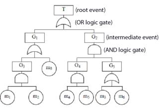
Fig. 3. An example of failure tree
