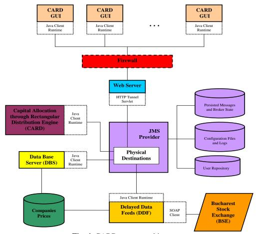
Fig. 4. CARD system architecture
